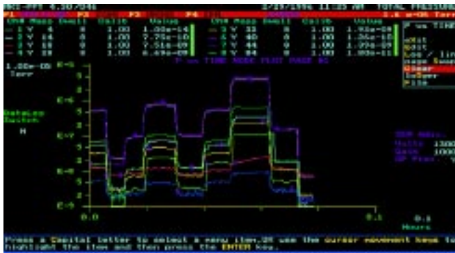
PPT for DOS provides Pressure vs. Time Mode that plots the partial pressure of up to 16 selected ions against time.
